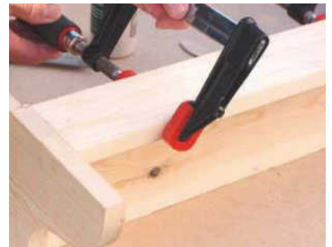
STEP 13. Upper and lower aprons are also fitted with biscuits. Sand the face sides before gluing in place
